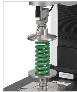
Compression spring testing
