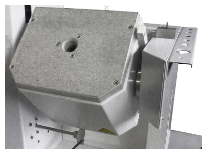
Tilting oven to facilitate cleaning of the chamber
