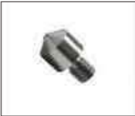
Φ1.588mm Carbide ball indenter
