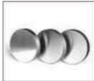
Rockwell Test block
