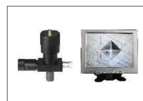
Vickers Video Measuring System (#823-811)
