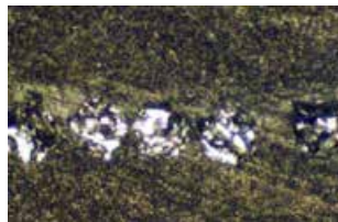
Boron-graphite composite sectioned with medium grit diamond wafering blade. Boron fibers damaged.
