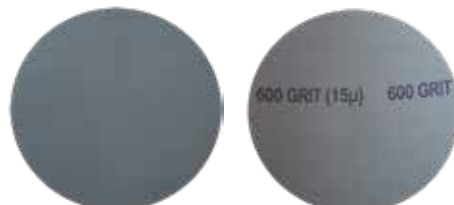
600 grit (15 micron) front / back side SiC foil
