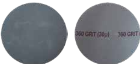
360 grit (30 micron) front / back side SiC foil
