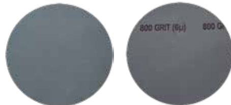
800 grit (6 micron) front / back side SiC foil
