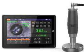
Brinell Measurement Software BrinScan
