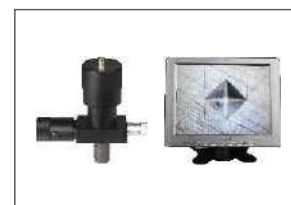
Vickers Video Measuring System (#823-811)
