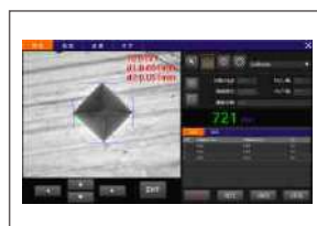
Vickers Measuring System (#821-834)
