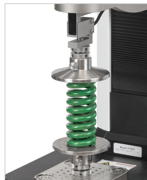
Compression spring testing
