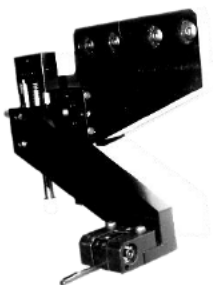
Micro-Force carbon Si Tun cantilever for contact fiber profilometry
