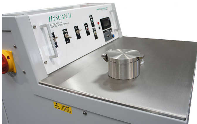
Hyscan II, used in production foundries worldwide, provides analysis within 5 minutes of sampling
